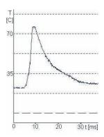
Fig. 3. Temperature inside the combustion chamber during compression process
